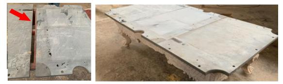
9. Use small gold wood screws to screw through predilled holes in slate into the wood of the base frame.
