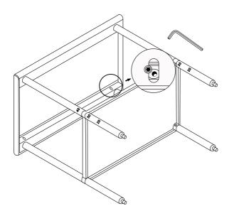
Step 3 Tighten the top plate screws.
