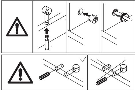
Attach panel 26 to panel 6 using wooden dowel(D), add cam lock(B) and turn clockwise to tighten.
