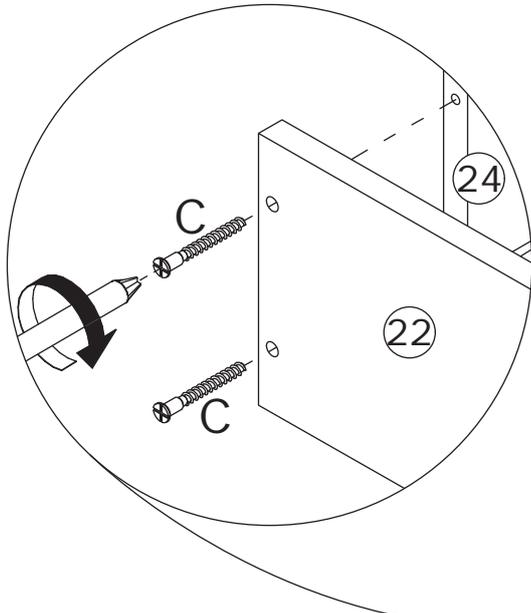
Attach panel 22 and panel 23 to panel 24 using screw(C) as shown.
