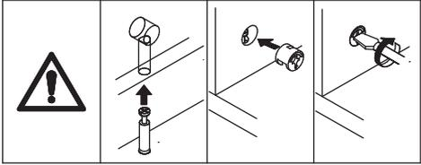
Attach panel 10 to panel 9, add cam lock(B) and turn clockwise to tighten.
