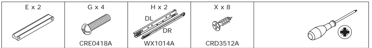
Attach handle(E) to panel 19 using screw(G).
