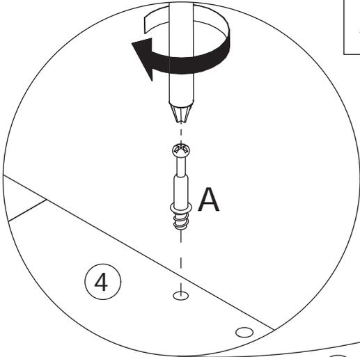
Screw the eccentric rod(A) into panel 4.
