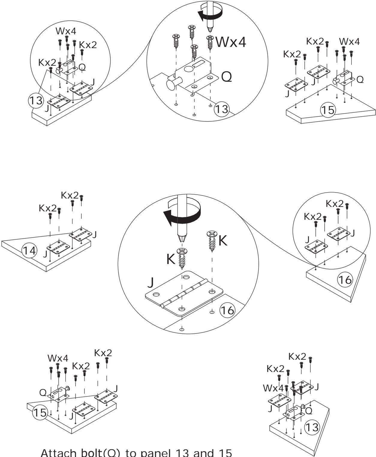
Attach bolt(Q) to panel 13 and 15 using screw(W) as shown.
