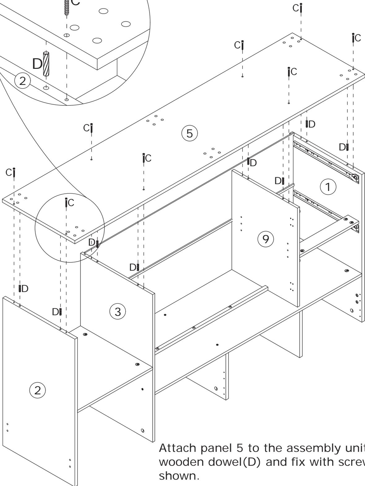
Attach panel 5 to the assembly unit using wooden dowel(D) and fix with screw(C) as shown.
