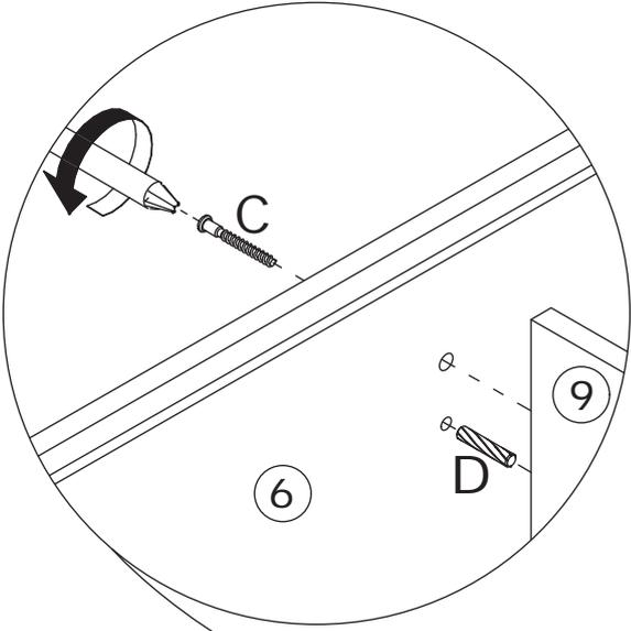
Attach panel 9 to panel 6 using dowel(D) and secure with screw(C) as shown.
