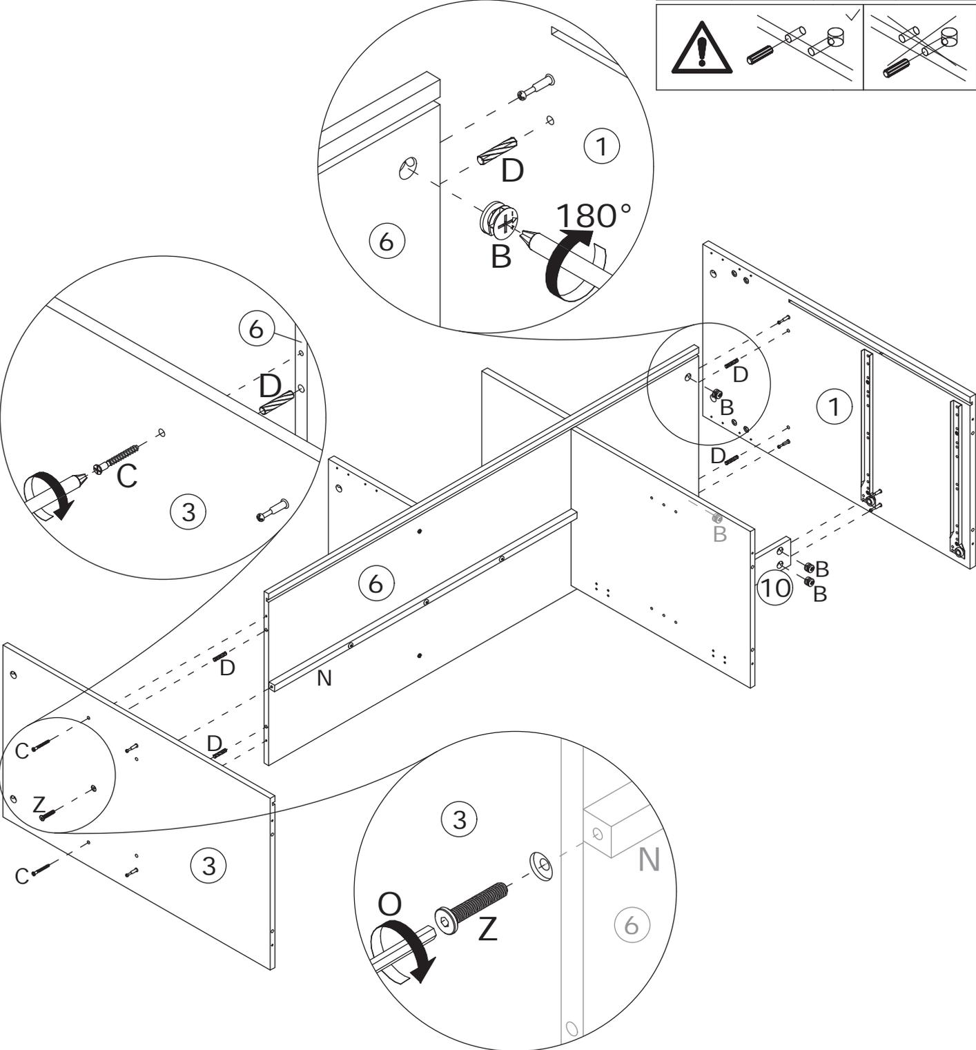
Attach panel 3 to panel 6 using wooden dowel(D) and fix with screw(C) as shown.
