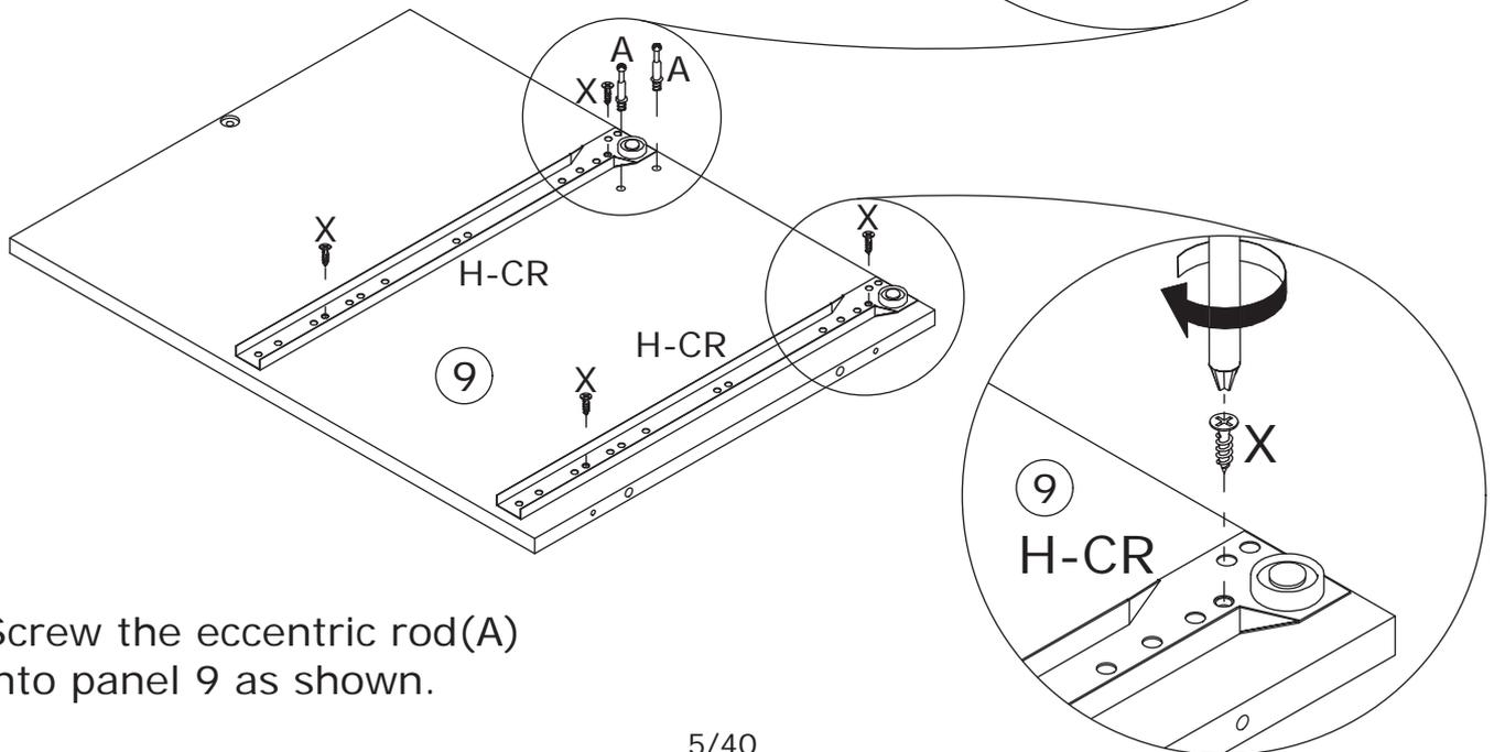
Screw the eccentric rod(A) into panel 9 as shown.
