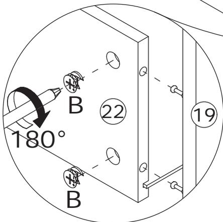
Attach panel 19 to panel 22 and 23, add cam lock(B) and turn clockwise to tighten as shown.
