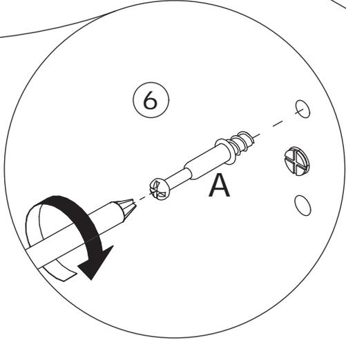
Fix panel 9 to tube(N) using screw(Z) as shown.
