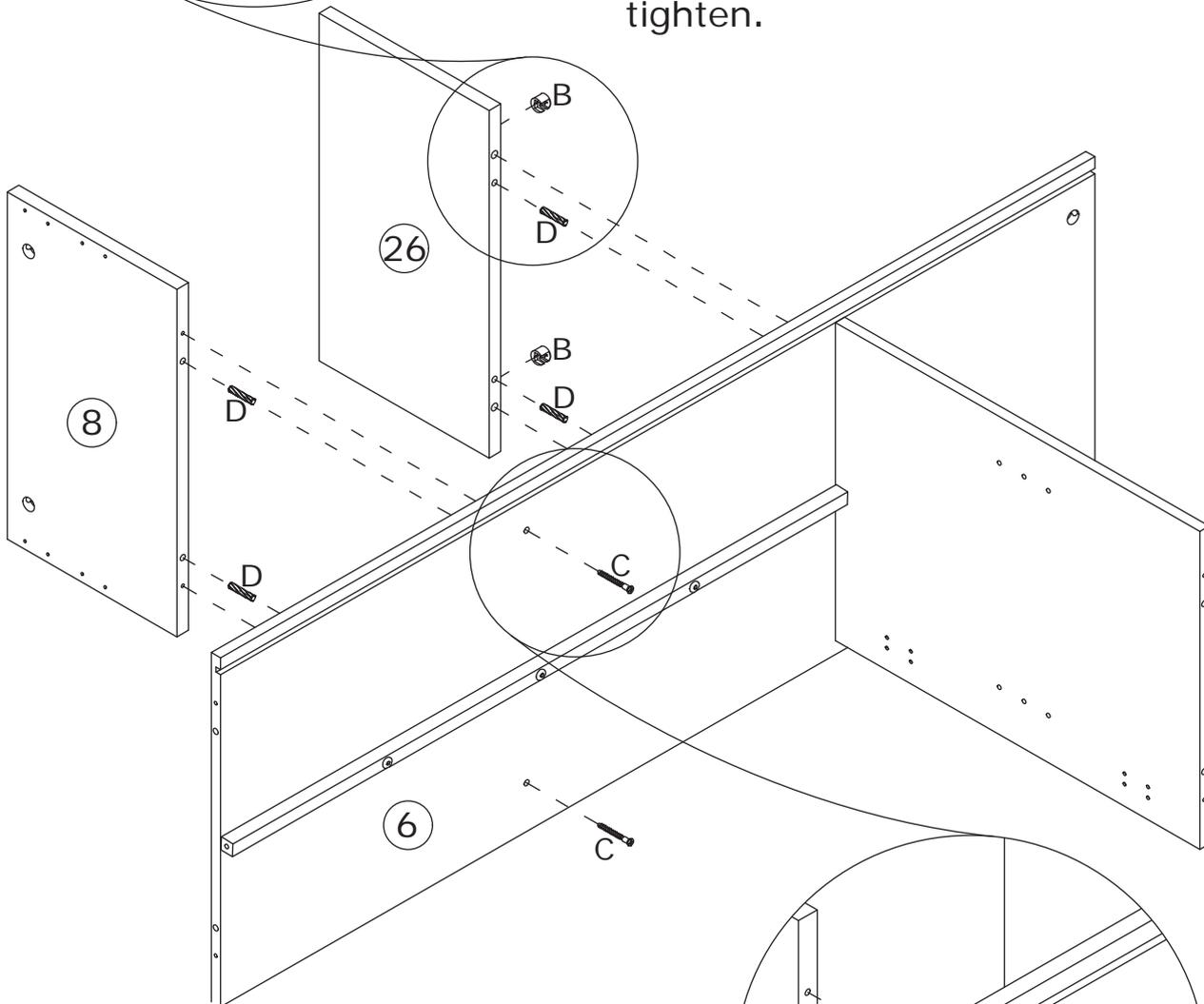
Attach panel 8 to panel 6 using wooden dowel(D) and fix with screw(C) as shown.
