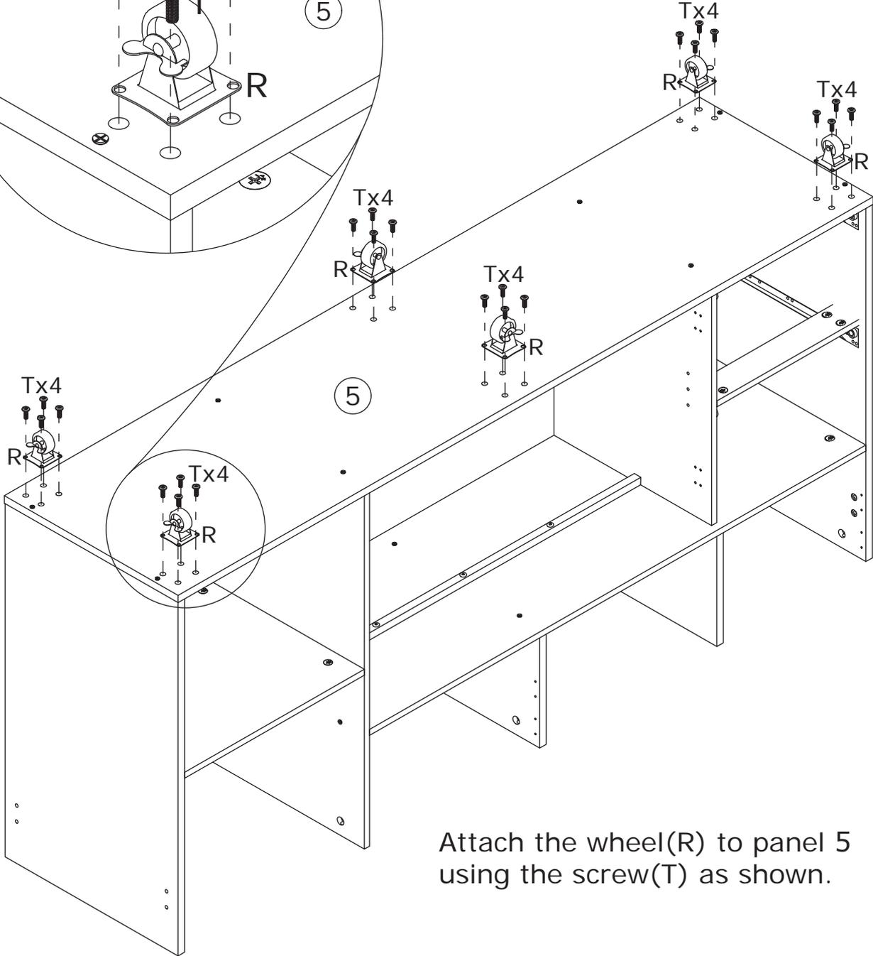
Attach the wheel(R) to panel 5 using the screw(T) as shown.
