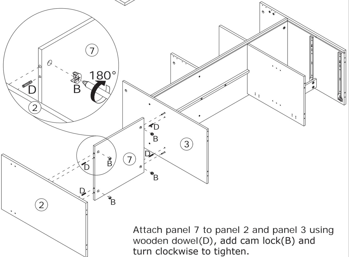
Attach panel 7 to panel 2 and panel 3 using wooden dowel(D), add cam lock(B) and turn clockwise to tighten.
