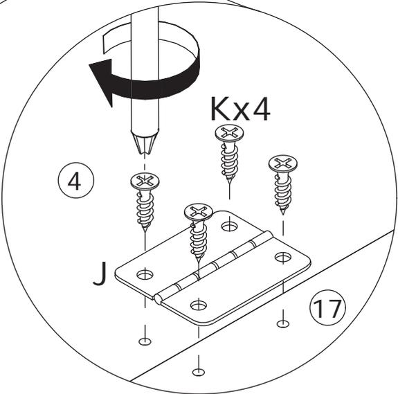
Attach panel 4 to panel 17 using hinge(J) and fix with screw(K) as shown.
