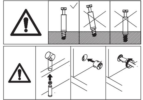
Screw the eccentric rod(A) into panel 19 as shown.
