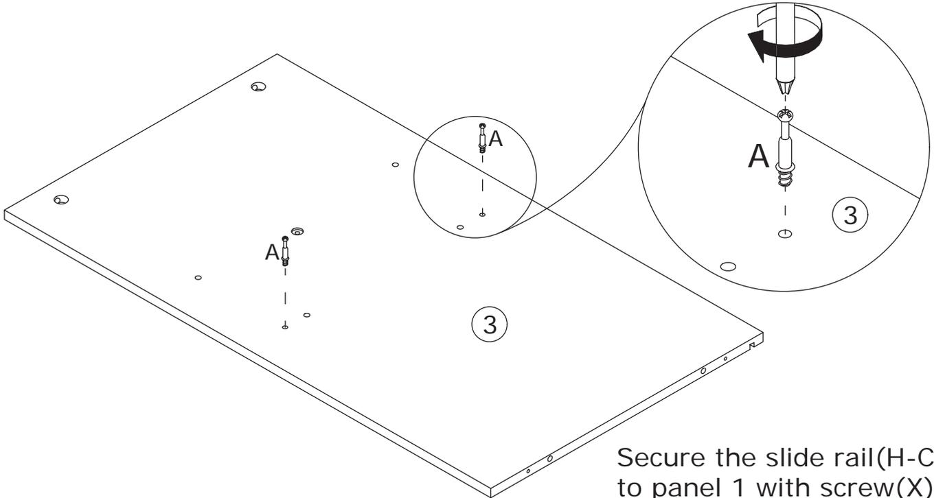
Secure the slide rail(H-CL) to panel 1 with screw(X) as shown.
