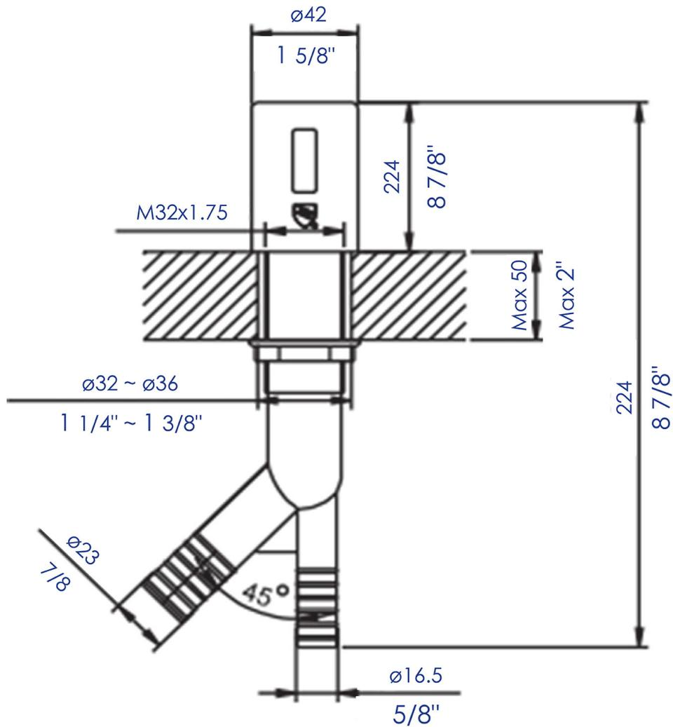
**Note:** All product dimensions are approximate and should be verified on site prior to installation.
