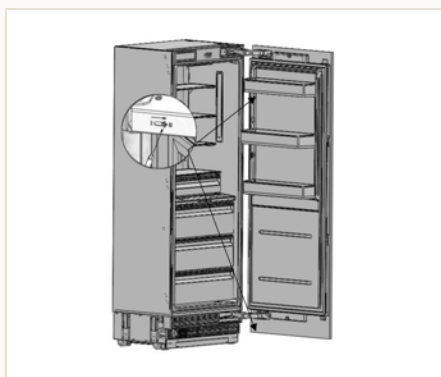
2 • REMOVE DOOR COVERS AND ADJUSTMENT KITS
