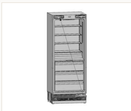
5 • MOVE HINGES AND HINGE CAPS ACROSS
