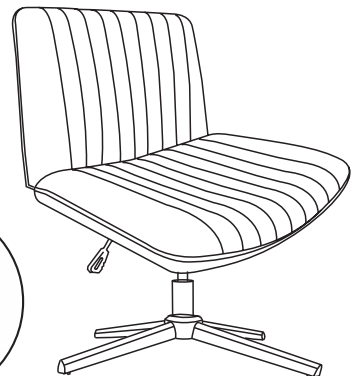
4.Rocking Adjustment Function The tighter the knob is turned, the less shaking it is, and vice versa
