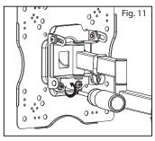
illustration using the screw driver (see Fig. 11). Rotate the screen until level and then re-tighten the safety screws. Never fully loosen or remove these screws.
