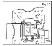
angle in place. Do not release the display until these screws are fully tightened and never fully loosen or remove these screws.
