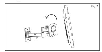
2 Replace the safety screws removed in preparation step and tighten.
