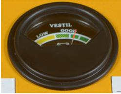
Always check the gauge before using the device; make sure that the battery is charged before using the stacker.
