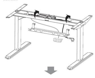
· Tighten all the screws on the hooks.
