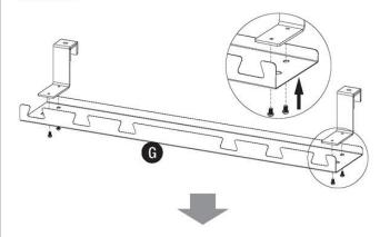
· Hang the cable management shelf onto the frame as shown below.
