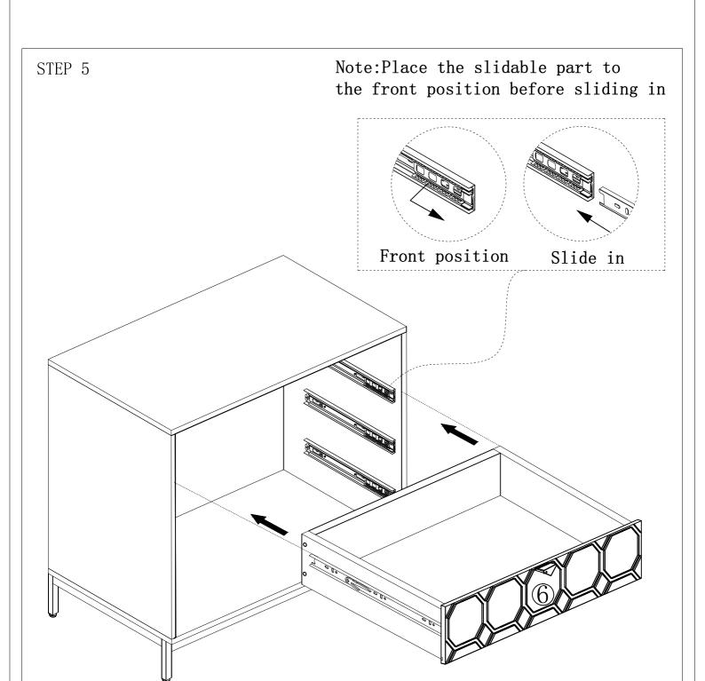
Reminder: If the front and both ends of the drawer are tilted, do not use force, You can refer to the above steps to smoothly insert the slide rail. The 6 # and 7 # and 8 # suction panels are not interchangeable
