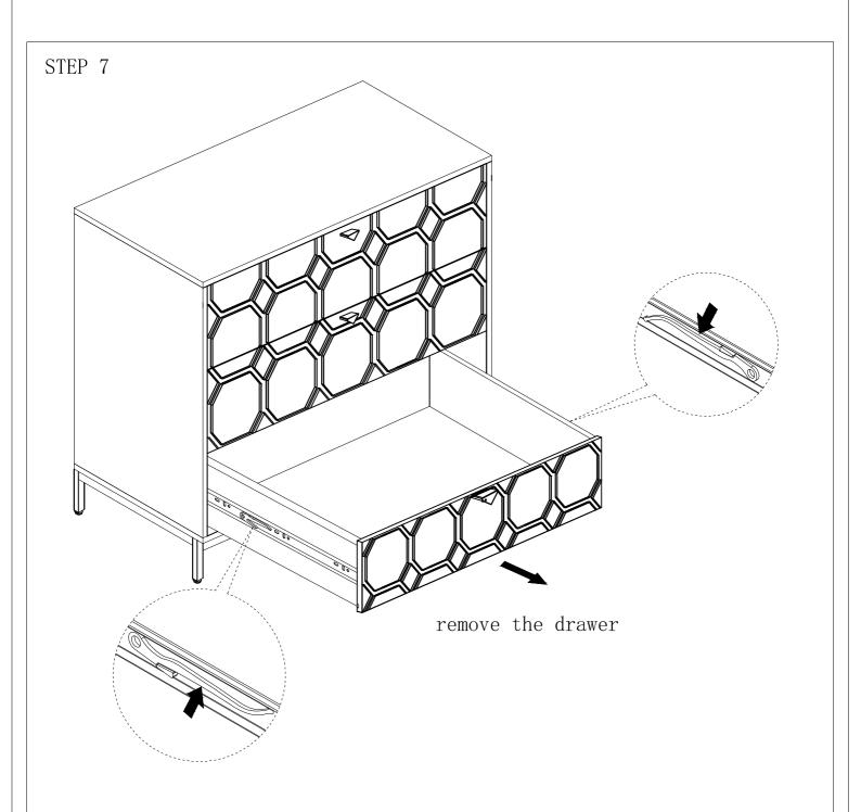
To remove the drawer. lift up on the left side buckleand press down on the right side buckle, operatingboth left and right at the same time, and move outward to remove it.
