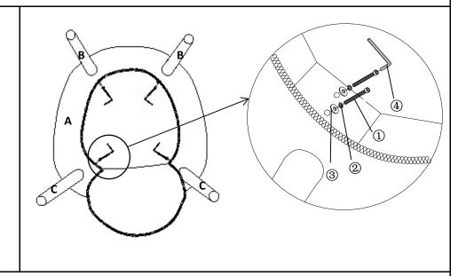
Insert the Back Leg(C) into the mounting position of Seat(A) and attach using Bolts(1), Spring Washers(2) and Washers(3) with Allen Key(4).
