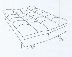
To release the supporting legs, please locate a release button on the top of the legs, press the button and fold the legs.
