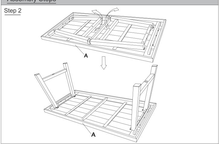
Place the Table (A) with the fabric face skywards onto a clean, soft surface to avoid any scratches or damages to the product.
