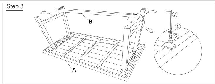
Attach the Leg Connector (B) to the Table(A).
