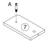
Fix screw(A) to board 3 and board 7 as shown.
