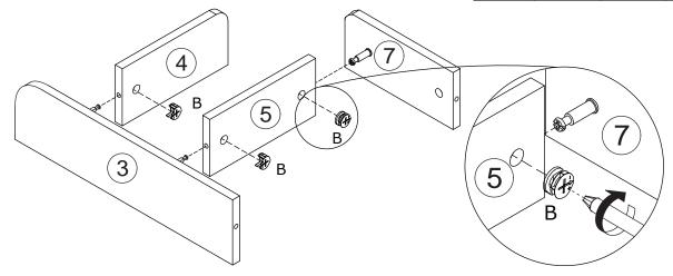
Connect board 3 and board 7 to board 4 and board 5, then insert cam lock(B) into board 4 and board 5 and tighten as shown.
