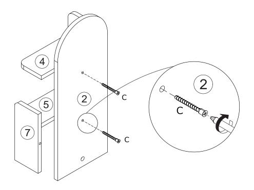
Connect board 2 to storage component using screw(C) as shown.
