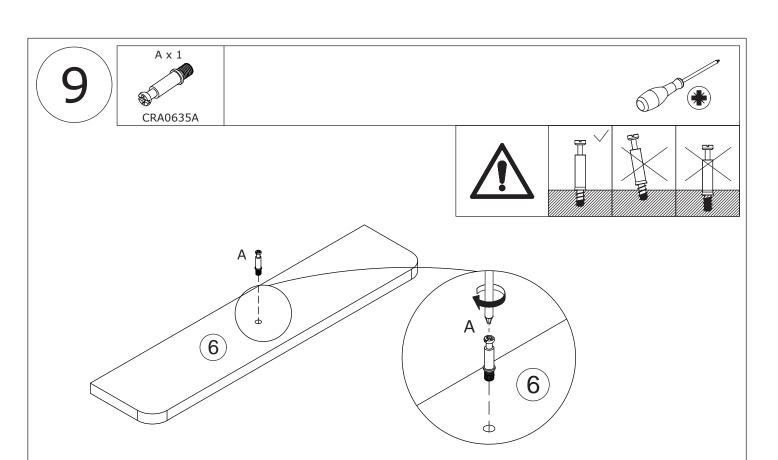
Fix screw(A) into board 6.
