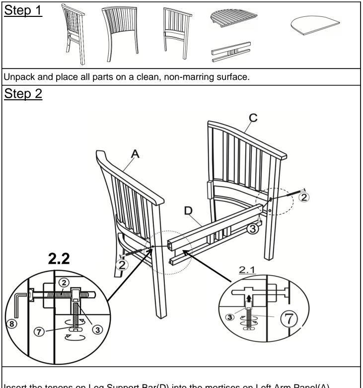
Insert the tenons on Leg Support Bar(D) into the mortises on Left Arm Panel(A). **2.1)** Insert Bolt((7)) into Cross Nut((3)), then insert the Cross Nut((3)) into the housing on Leg Support Bar(D) as shown above.
