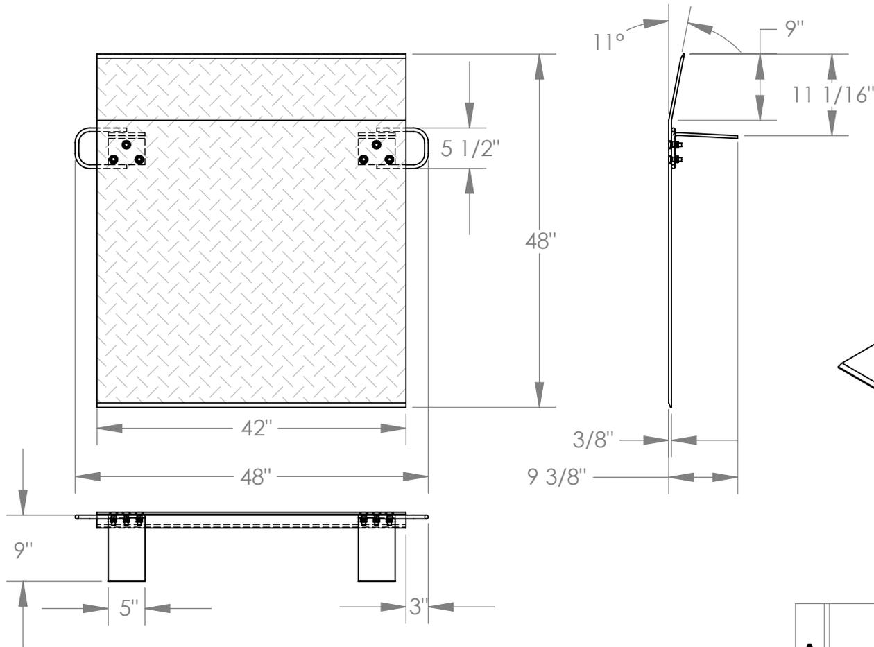
NOTE: BEND OR CROWN IS 11° AND LOCATED 9" FROM EDGE OF DOCKPLATE
