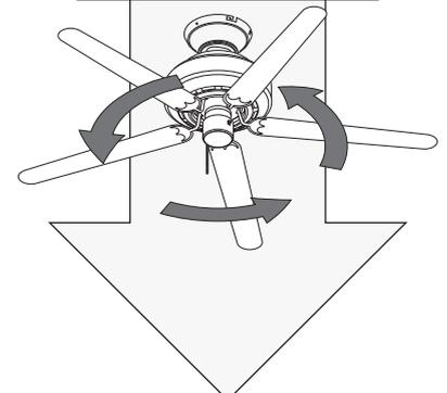
Downdraft (counterclockwise rotation) creates a direct breeze and maximum cooling effect.
