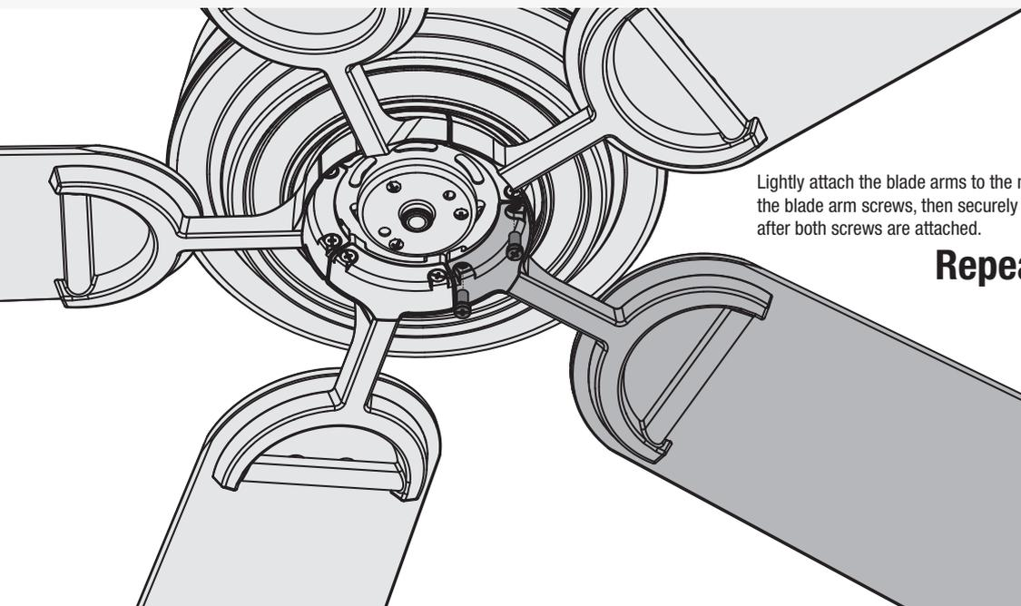
Lightly attach the blade arms to the motor with the blade arm screws, then securely tighten after both screws are attached.
