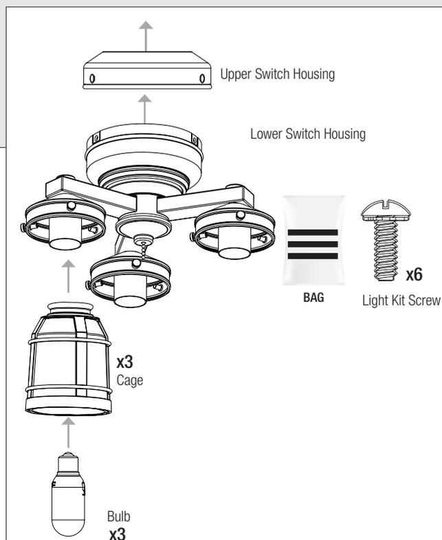
For installing the light fixture
