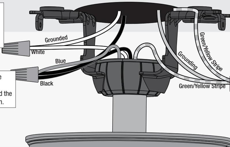
Connect the black wire (ungrounded) from the ceiling to the black and the blue wires from the fan.
