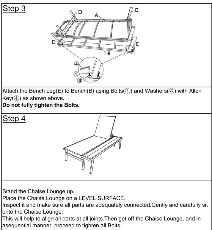
When tightening the Bolts, tighten sequentially.
