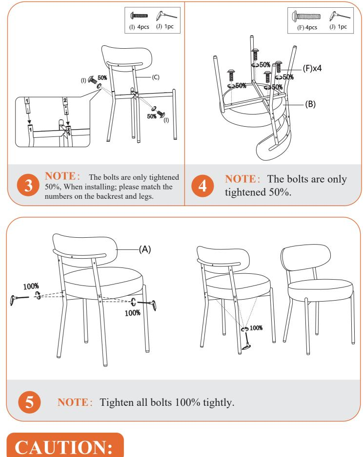
\* Before using the chair, check to ensure that all bolts are fully tightened. \* Lubricate all parts and tighten all bolts every 6 months or whenever needed. **NOTE**: 1. All bolts are 100% tightened.
