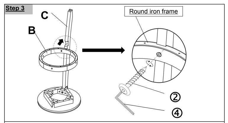
Insert Foot support frame (B) into the leg (C), using screw (②) as above picture. Affix Foot support frame (B) and leg (C) by using Allen key (④). **Do not fully tighten the Bolts.**
