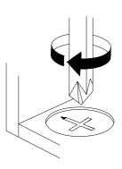
Turn cam lock clockwise to tighten.
