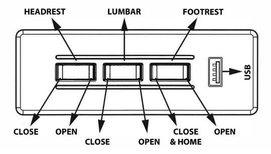
**To recline:** Sit on the furniture, and press the front of the button closest to the footrest to smoothly raise the footrest and recline to any position. To lower the footrest and return to an upright position, press the back side of the button closest to the footrest.
