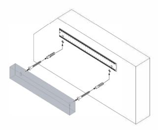
**Wall fixings:** Because of the variety of different wall types, We cannot provide you with an exact fixing you will need to fix this product to the wall. You must first identify the type of the wall you intend to fix product onto and then contact your local hardware store to get appropriate fixings.
