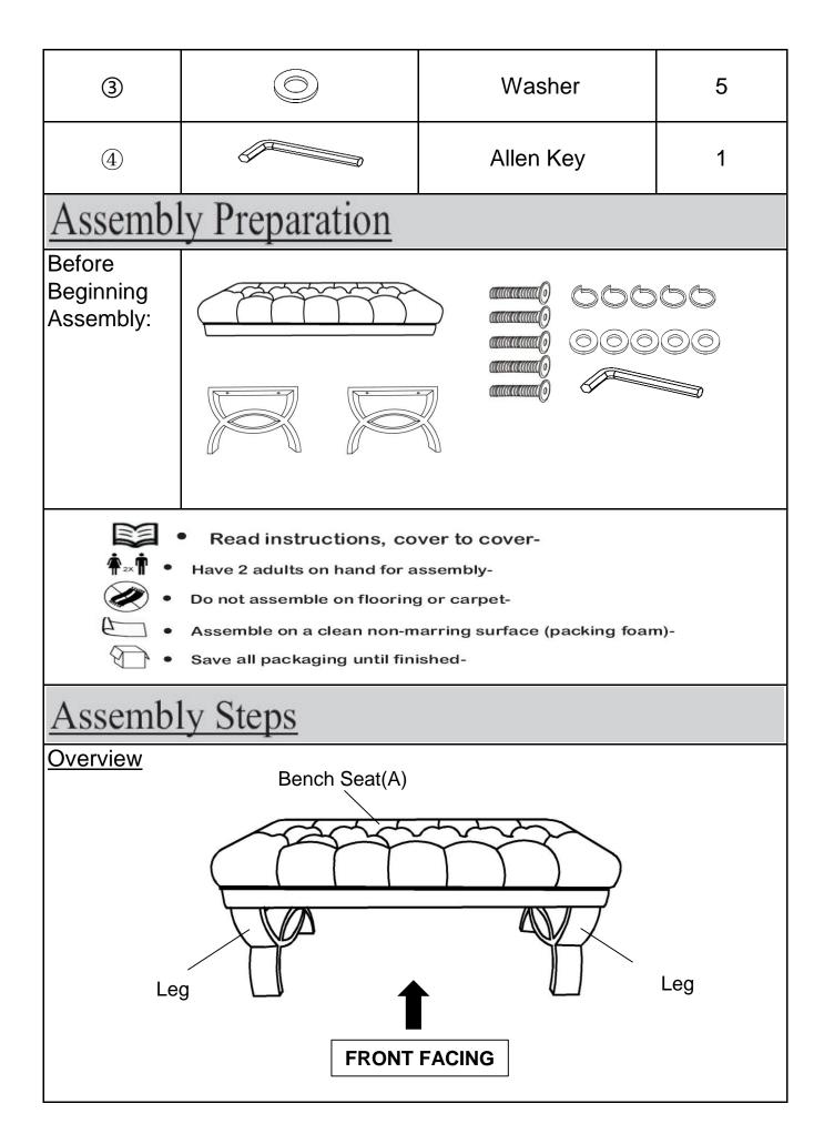
This Bench has multiple parts and may require up to 30 minutes to assemble. To give you an overview of the Bench parts, the above picture is to help you put the various parts into perspective. Please read through the instructions below to familiarise yourself with the parts and steps before assembly.
