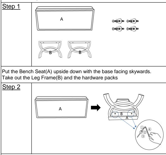
Align the mounting positions on the Leg Frame(B) to those on the underside of Bench Seat(A).
