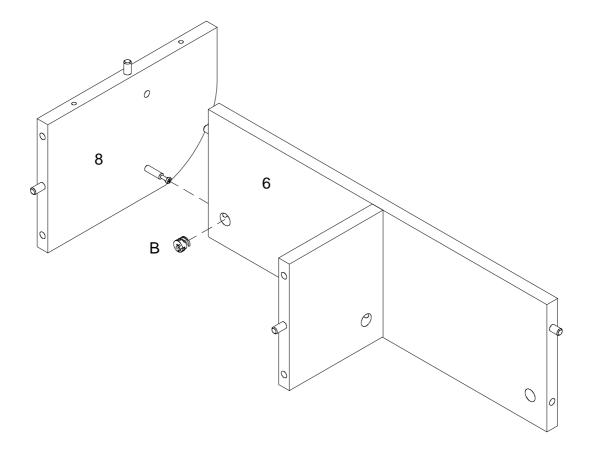
Using cam lock (B) secure part (8) into part (6) with Philips Head screwdriver as per diagram.
