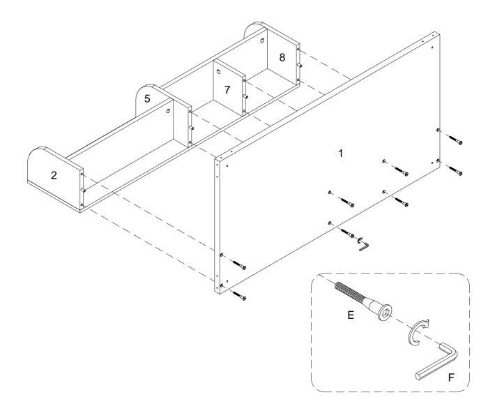
Using bolt (E) secure part (1) into parts (2,5,7,8) with hex key (F) as per diagram.
