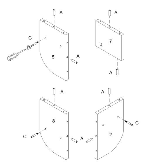
Insert wooden dowel (A) into parts (2,5,7,8), using cam bolt (C) secure parts (2,5,8) with Philips Head screwdriver as per diagram.
