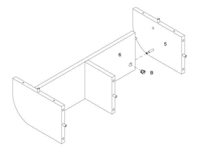
Using cam lock (B) secure part (5) into part (6) with Philips Head screwdriver as per diagram.
