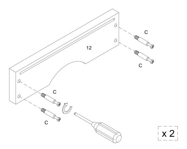
Using cam bolt (C) secure part (12) with Philips Head screwdriver as per diagram.
