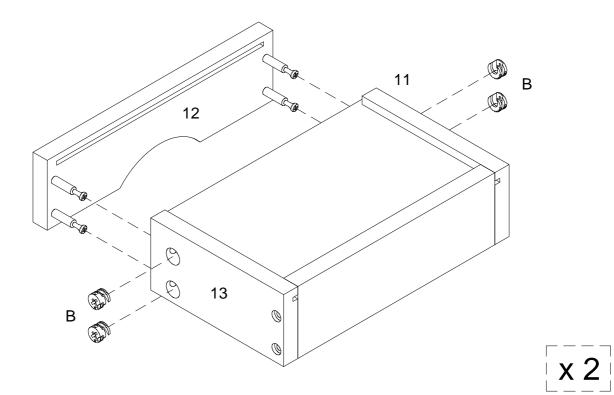
Using cam lock (B) secure part (12) into parts (11,13) with Philips Head screwdriver as per diagram.
