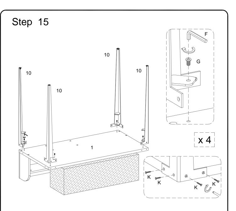
Using bolt (G) secure part (10) into part (1) with hex key (F) ,and using screw (K) secure part (10) into part (1) with Philips head screwdriver as per diagram.
