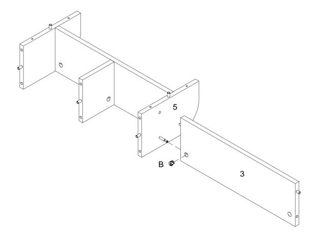
Using cam lock (B) secure part (3) into part (5) with Philips Head screwdriver as per diagram.
