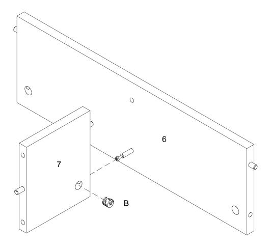
Using cam lock (B) secure part (7) into part (6) with Philips Head screwdriver as per diagram.
