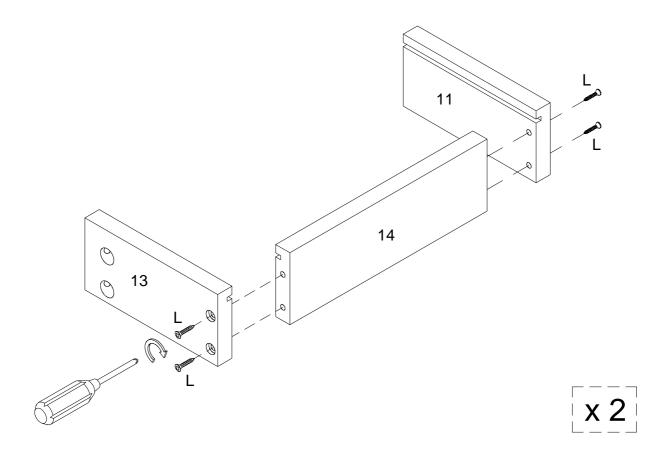
Using cam screw (L) secure parts (11,13) into parts (14) with Philips Head screwdriver as per diagram.
