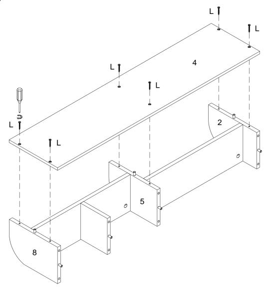
Using screw (L) secure part (4) into parts (2,5,8) with Philips Head screwdriver as per diagram.
