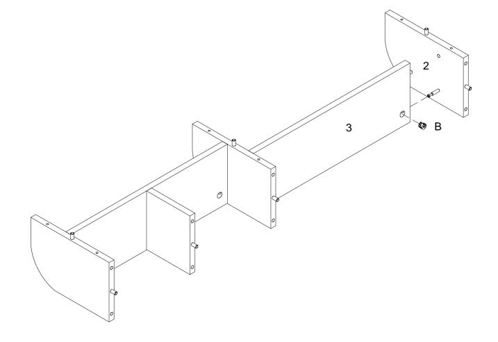
Using cam lock (B) secure part (2) into part (3) with Philips Head screwdriver as per diagram.
