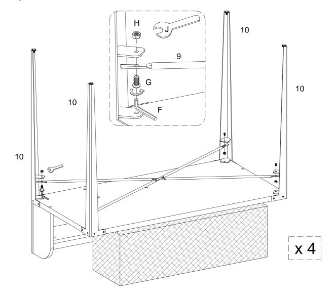
Using bolt (G) secure part (9) into nut (H) to part (10) with wrench (J).
