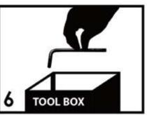
Save the instructions and store any supplied tool for later maintenance. After two weeks, check and tighten any loose hardware and repeat again every six months thereafter.
