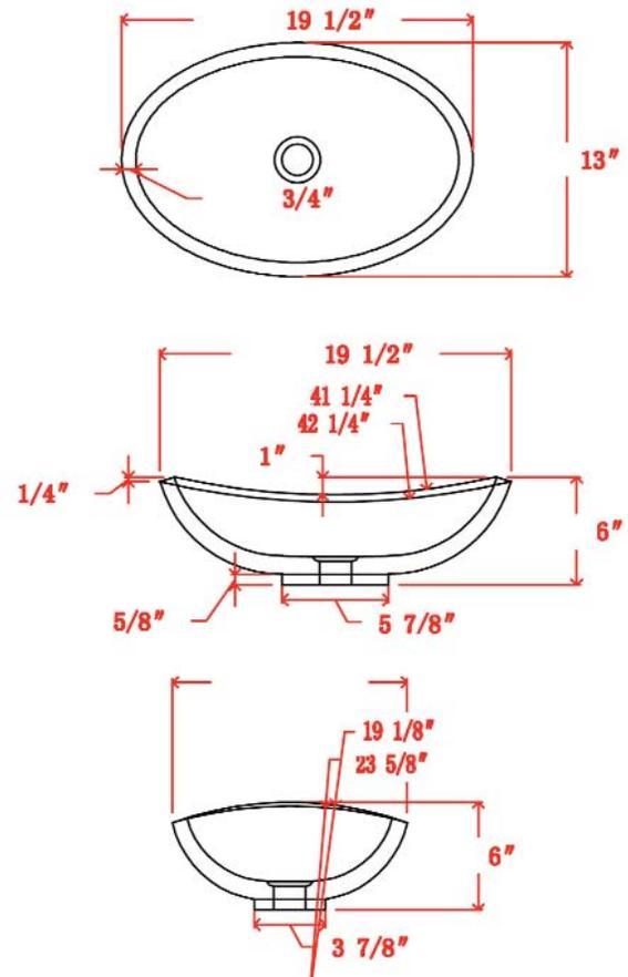
Dimensions of fixture are nominal and may vary within the range of tolerances established by ASME Standard A112.19.2. Dimensions and specifications subject to change without notice.
