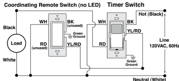
**WIRING COORDINATING REMOTE SWITCH (VP0SR-10): Connect wires per WIRING DIAGRAM as follows:**
