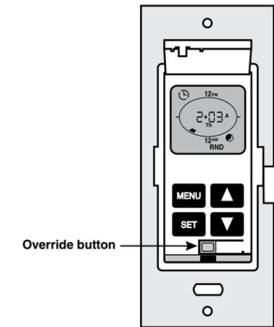
b) Press and hold **SET** followed by (**Override**) until **DEL** stops flashing and **5-0** flashes (approximately 5 seconds). Press **SET** to confirm device **Reset**.
