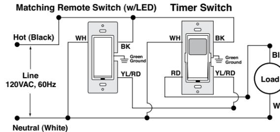
**NOTE:** The timer switch **must** be installed in a wall box that has a Load connection. The matching remote **must** be installed in a wall box with a Line Hot connection and a Neutral connection. A Neutral wire to the matching remote needs to be added as shown.
