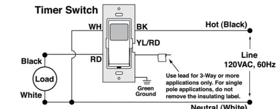
**WIRING TIMER SWITCH: Connect wires per WIRING DIAGRAM as follows:**
