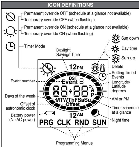
**Timer Schedule at a Glance** will allow you to quickly see your timers ON/OFF settings for the day. The displayed segments represent the time(s) your load will be on. The segment representing the current time will be flashing.
