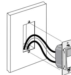
**NOTE:** Dress wires with a bend as shown in diagram in order to relieve stress when mounting device.
