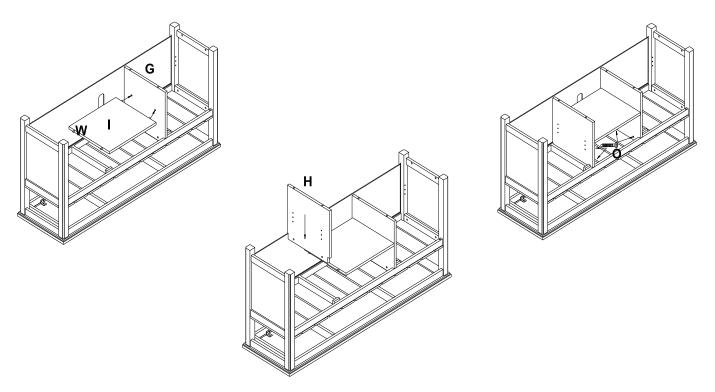
Attach Bottom (E) to Side Assemblies using 4-35MM Hex Bolts. Attach Bottom (E) to Vertical Dividers using 4 - 30MM Hex Bolts (O). Attached Center Post (M) by threading it in to insert on undside of Botom Panel (E). **NOTE: AT THIS TIME TIGHEN ALL HEX BOLTS.**
