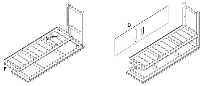
Attach Side Assembly (C) to Top Assembly and Slat Shelft (A & F) using 4-35MM Hex Bolts (N). **NOTE: DO NOT TIGHEN FIRMLY AT THIS TIME.**
