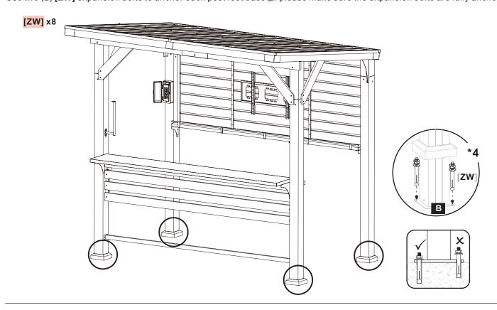
Outdoor Structure anchoring guide for anchoring gazebo to wood or concrete: If step 43, on page 26 in the assembly instructions is not properly completed, this will void the warranty.
