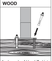
Anchors should be drilled into joists or reinforced blocking (not only deck boards).
