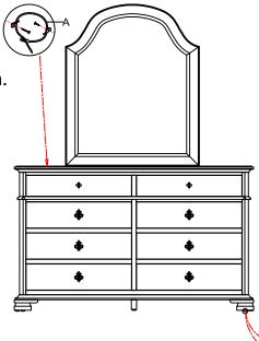
Adjust Leveler if needed to level case on uneven floor.
