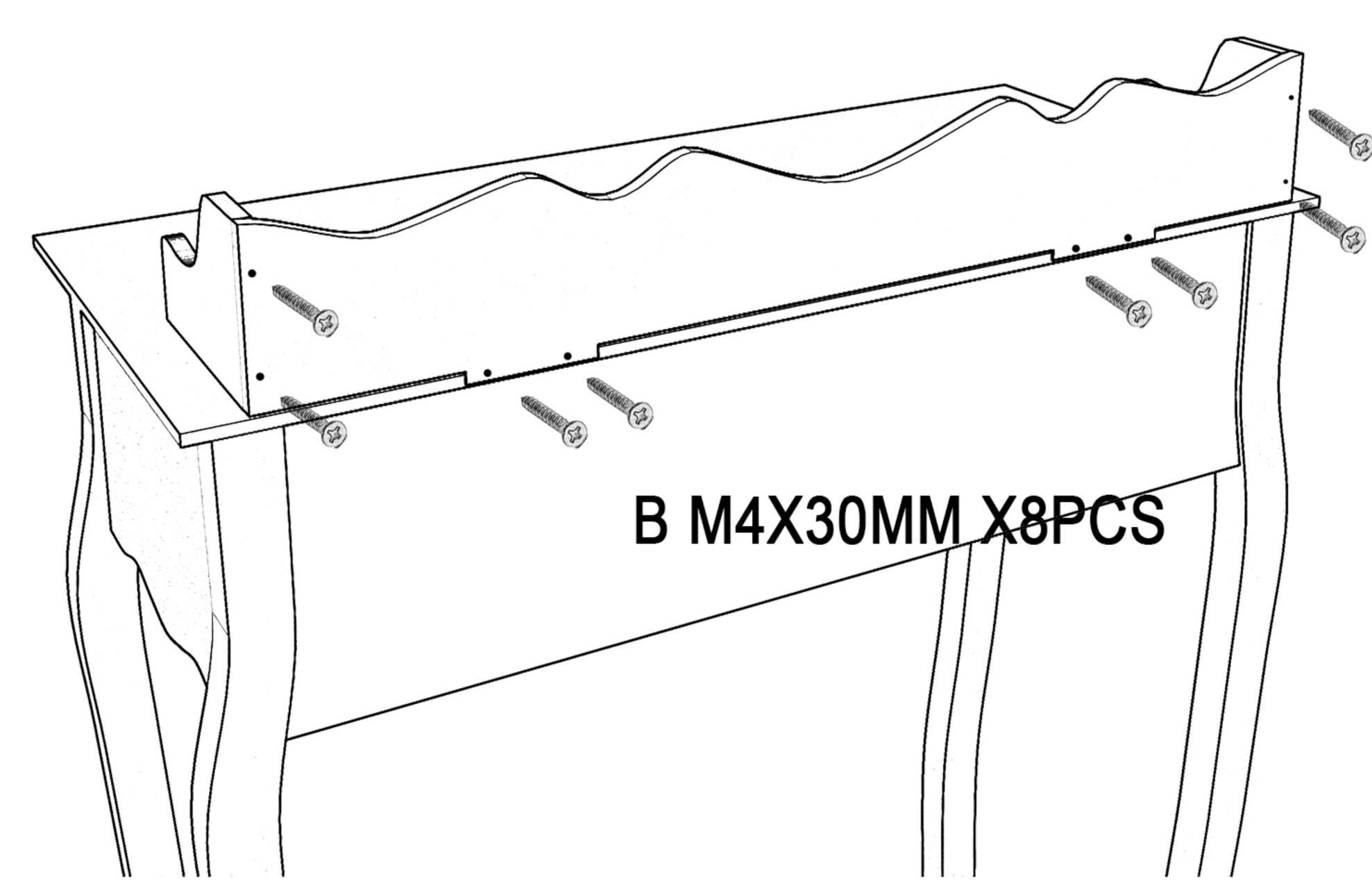
USE HARDWARE A(X8PCS) TO CONNECT THE TAILGATE, SIDE FENCE AND DESKTOP TOGETHER.
