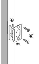
Mount the strike onto the door frame by aligning it with the latch height before drilling the required holes.
