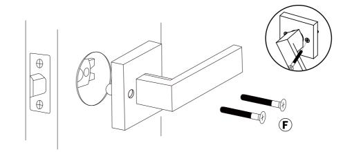
Attach the indoor handle lock to the square bolt on the outside and align the screws from the interior latch towards the posts.
