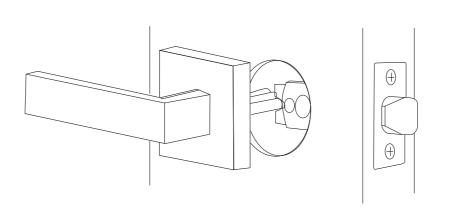
Secure the exterior handle lock in position by inserting the posts and square bolt into the latch mechanism holes.
