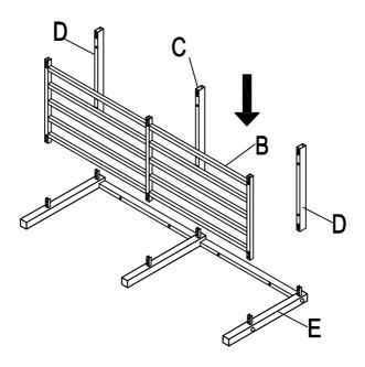
Attach the Front Frame (E) to the Middle Top Iron Stretcher (C), Two Sides Top Iron Stretcher (D) and Bottom Frame (B).
