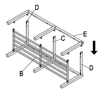
Attach the Bottom Frame (B) and Two Sides Top Iron Stretcher (D) to the Front Frame (E) by using Flat Washer (H), Lock Washer (G) and Bolt (F) with Allen Key (I).
