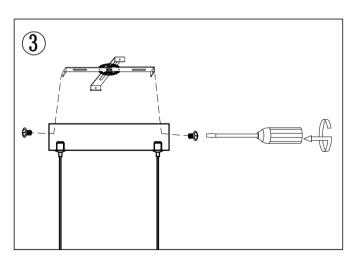
3. Install the ceiling pan with the wall-mount plate on the ceiling by using screws as drawing ③ showing.
