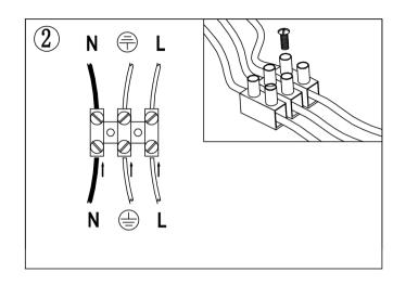
2. Connect the electronic wire as drawing ② showing.
