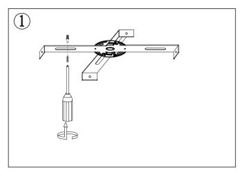
1. Install the ceiling-mount plate on the ceiling by using screws as drawing ① showing.
