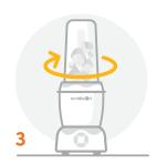
Turn the cup upside down and place it onto the motor base, gently turning clockwise to lock in place.
