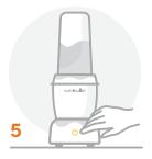
When ready, stop the appliance by pressing POWER (), or the function that's running, and wait for blades to stop turning.
