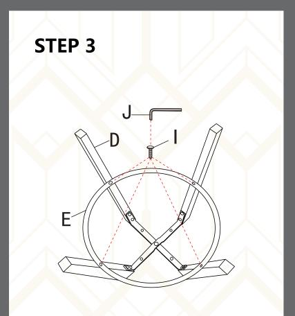
Twist Screw (I) to the (E) with (D) . Then tighten (I), (G) and (H) completely.
