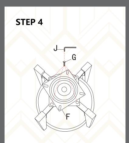
Rotate (F) 45 ° as displayed. Twist Screw (G) to the (F) with (B) and (C).
