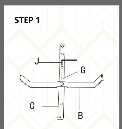
Place (B) on (C) as displayed, then twist Screw (G) to connect them. Only twist (G) into half way.
