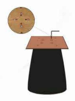
③ Place the connecting plate on the base and secure the connecting plate and base with screws.
