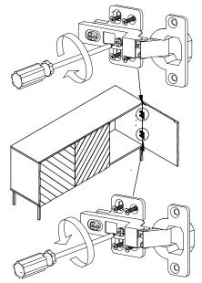
Turn left middle bolt adjuster properly until door is balanced
