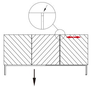
Turn right middle bolt adjuster properly until door is balanced
