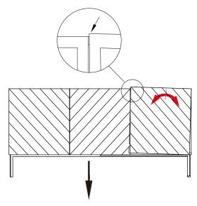
Turn right middle bolt adjuster properly until door is balanced
