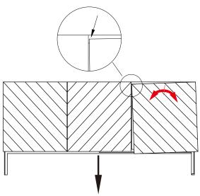
Turn left middle bolt adjuster properly until door is balanced
