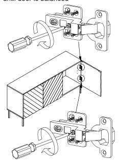
Turn right middle bolt adjuster properly until door is balanced
