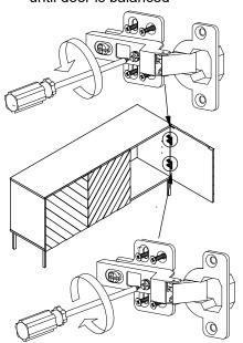
Turn right middle bolt adjuster properly until door is balanced
