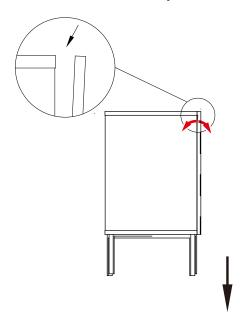
Turn left the adjuster properly until door is balanced
