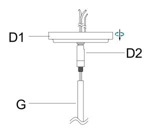
then cut off the extra cord so that 6" wires at least long within the outlet junction box.
