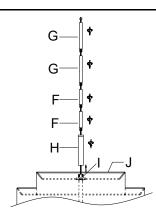
Step 2:Insert the power cord through Lower tube (H), Short tube (F) and Long tube (G) as desired length. Insert the Lower tube (H) into the center threaded portion (I) of the Shade(J) until tight. Rotate each tubes clockwise till tight.
