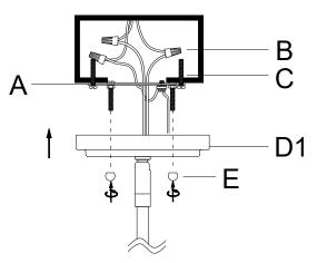
**Step 6:**Raise the Canopy (D1) over the Mounting Plate (A), making sure 2 Threaded Rods extend downwards through 2 holes on the Canopy (D1). Secure the Canopy (D1) by turning the Canopy Nuts (E) clockwise until tight.
