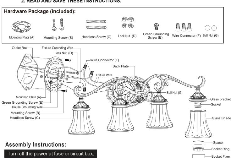
1. Thread two headless screws through the mounting plate, then secure them with four lock nuts (two on each side of the mounting plate). Adjust the length of the headless screws if necessary.
