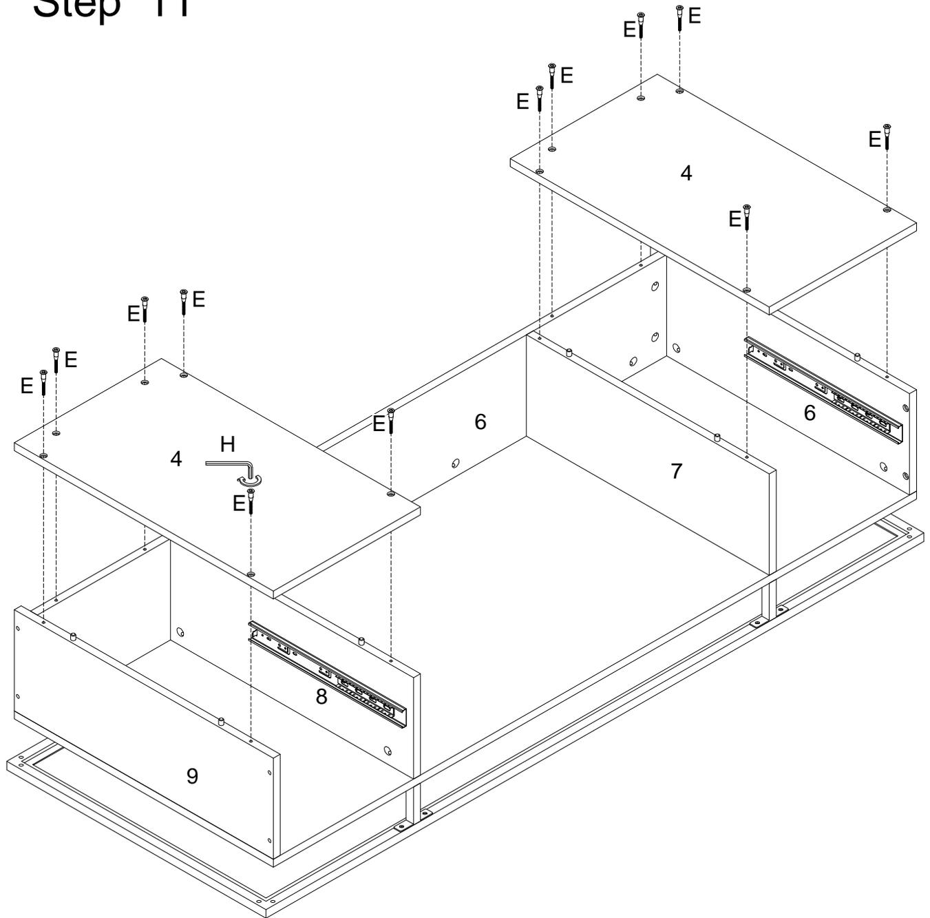
Using screw (E) attach part (4) into parts (6,7,8,9,10) with hex key (H) as per diagram.
