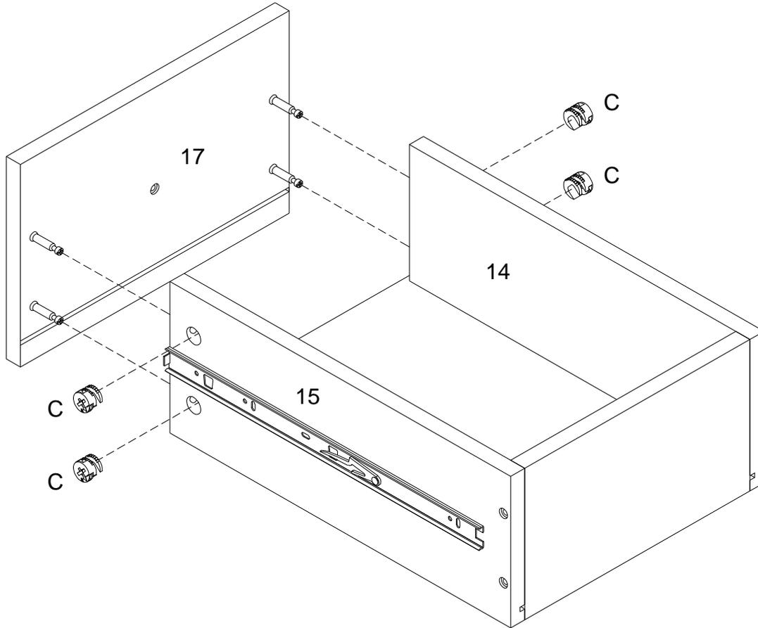
Using cam lock(C) secure part (17) into parts (14,15) with Philips head screwdriver as per diagram.
