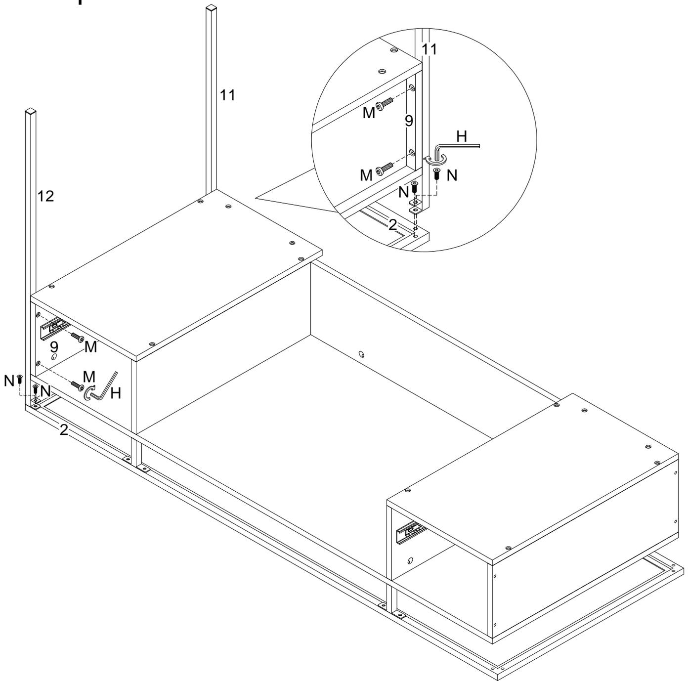
Using bolts (M,N) attach parts (11,12) into parts (2,9) with hex key (H) as per diagram.
