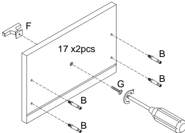
Secure cam bolt (B) into part (17), then using bolt (G) attach handle (F) into part (17) and using screw (L) attach slider (Q) into parts (14,15), with Philips head screwdriver as per diagram.
