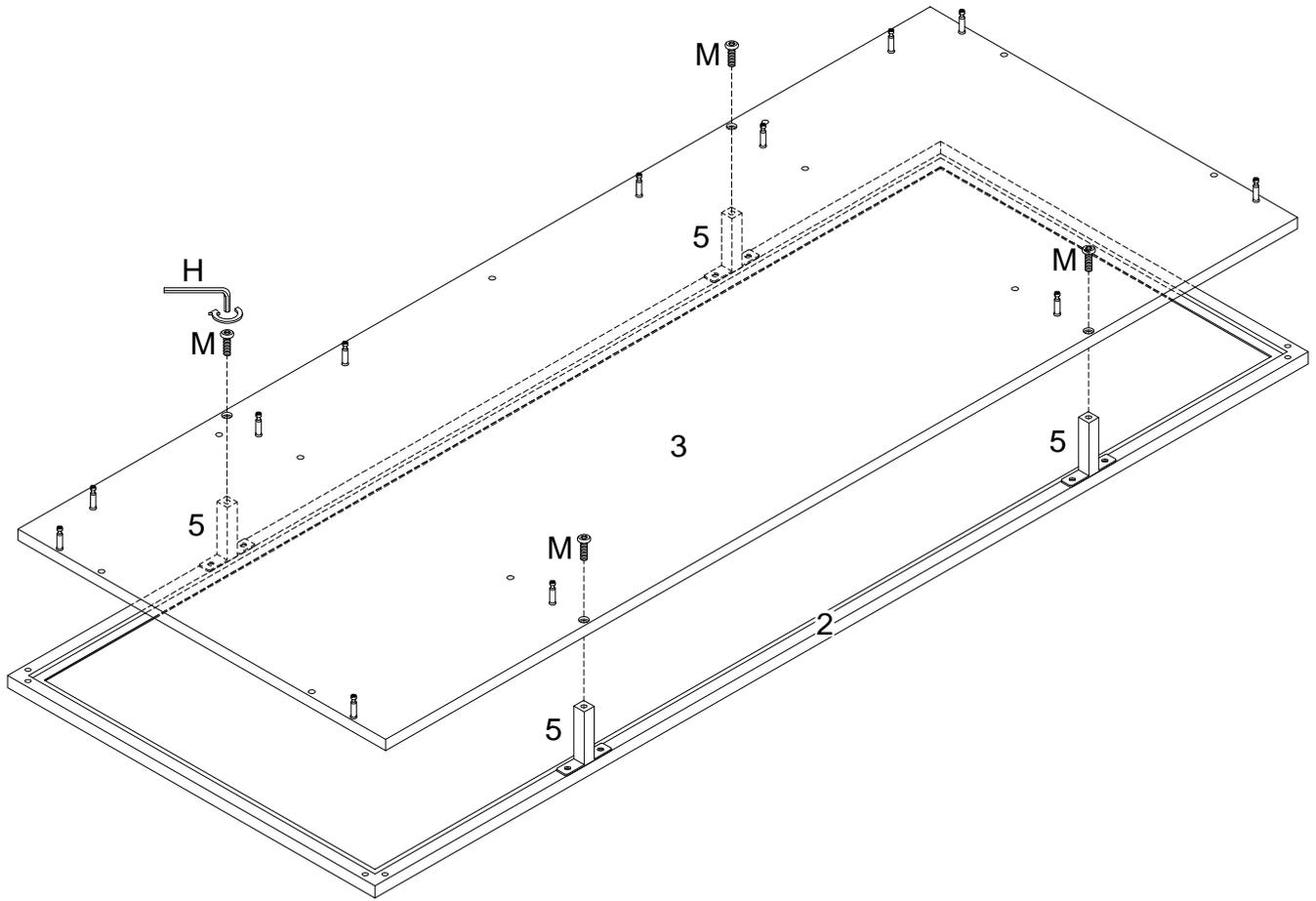
Using bolt (M) attach part (3) into part (5) with hex key (H) as per diagram.
