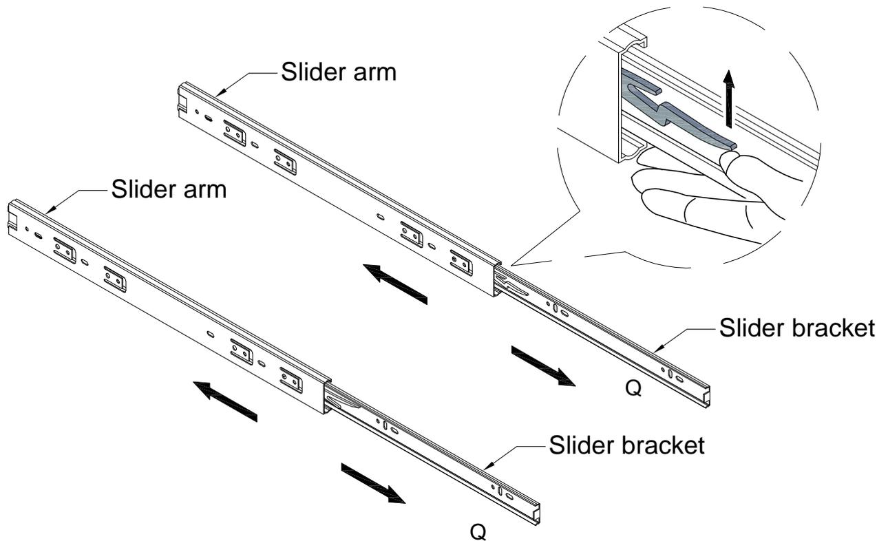
Pick up the Ball Bearing Slides (Q) and separate the slide Runner for the following Steps. Extend the Slide Runner all the way forward, press the plastic release lever of the ball bearing Slides up and pull the Slide Runner Complete out .
