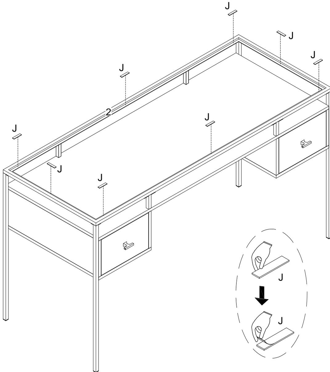
Tear off and put glass pads (J) as per diagram.
