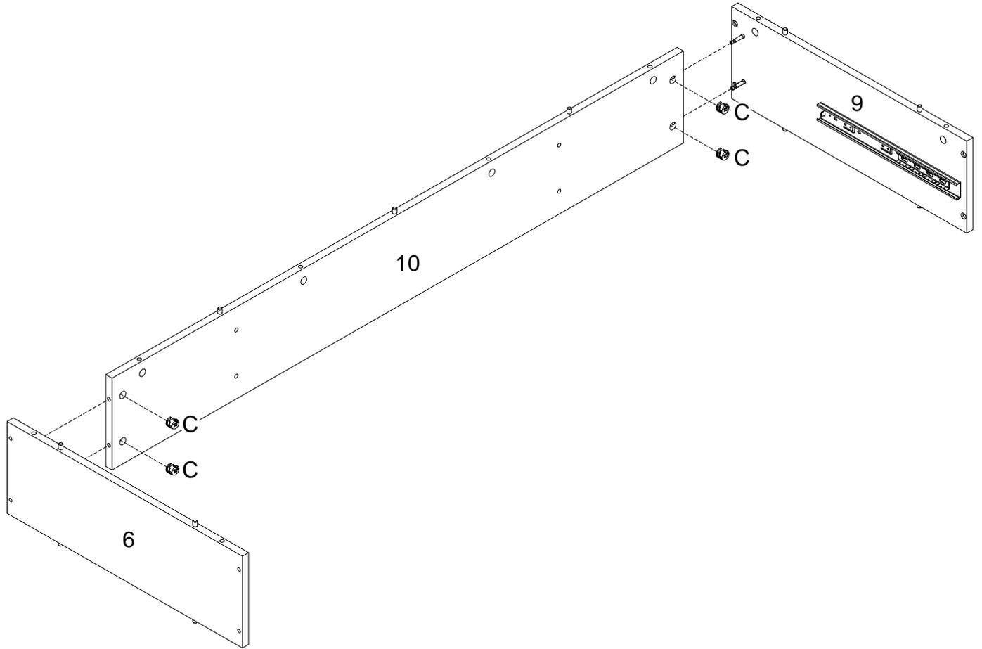
Using cam lock(C) secure parts (6,9) into part (10) with Philips head screwdriver as per diagram.
