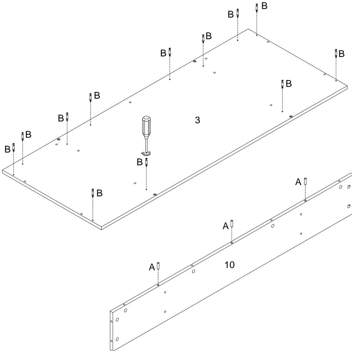
Insert wooden dowel (A) into part (10) ,then secure cam bolt (B) into part (3) with Philips head screwdriver as per diagram.
