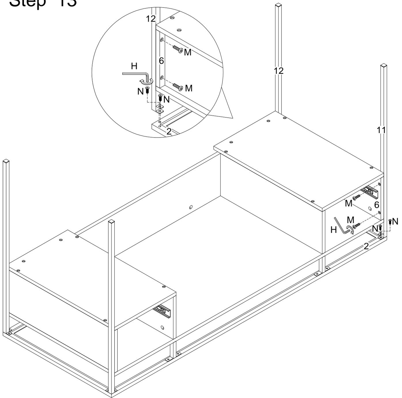
Using bolt (M,N) attach parts (11,12) into parts (6,2) with hex key (H) as per diagram.
