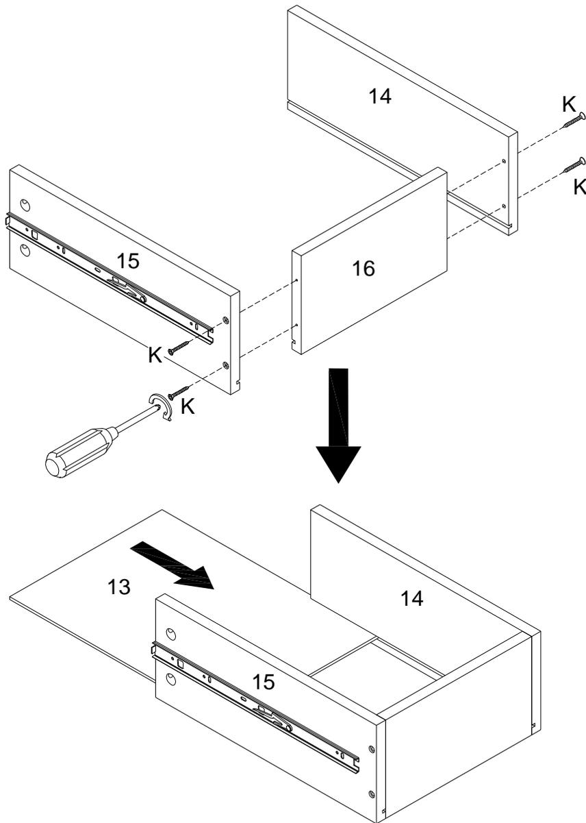
Using screw (K) attach parts (14,15) into part (16) with Philips head screwdriver ,then put part (13) as per diagram.
