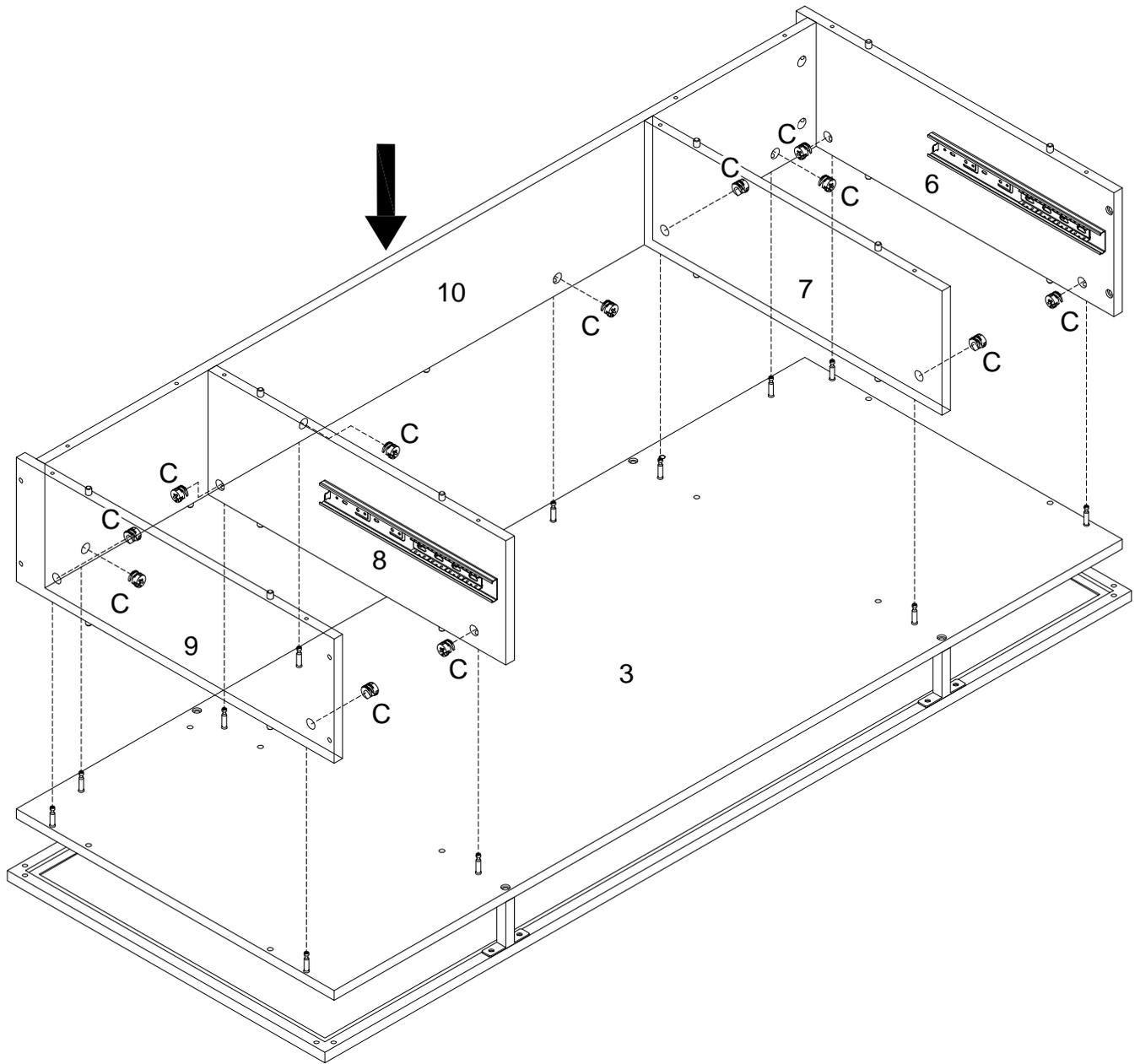
Using cam lock(C) secure parts (6,7,8,9,10) into part (3) with Philips head screwdriver as per diagram.
