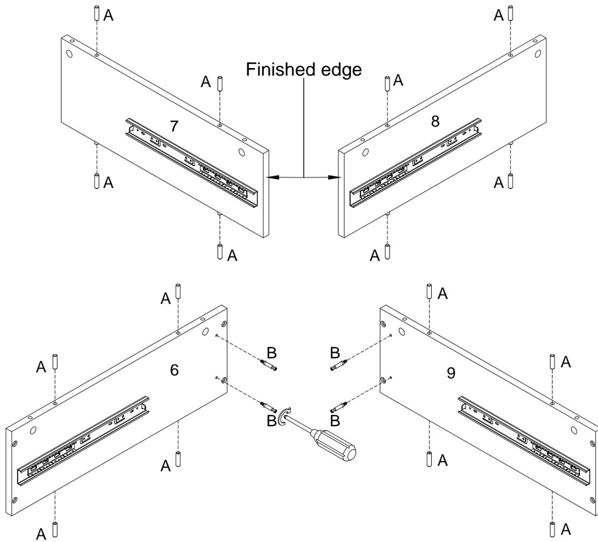
Insert wooden dowel (A) into parts (6,7,8,9,) ,then secure cam bolt (B) into parts (6,9) with Philips head screwdriver as per diagram.
