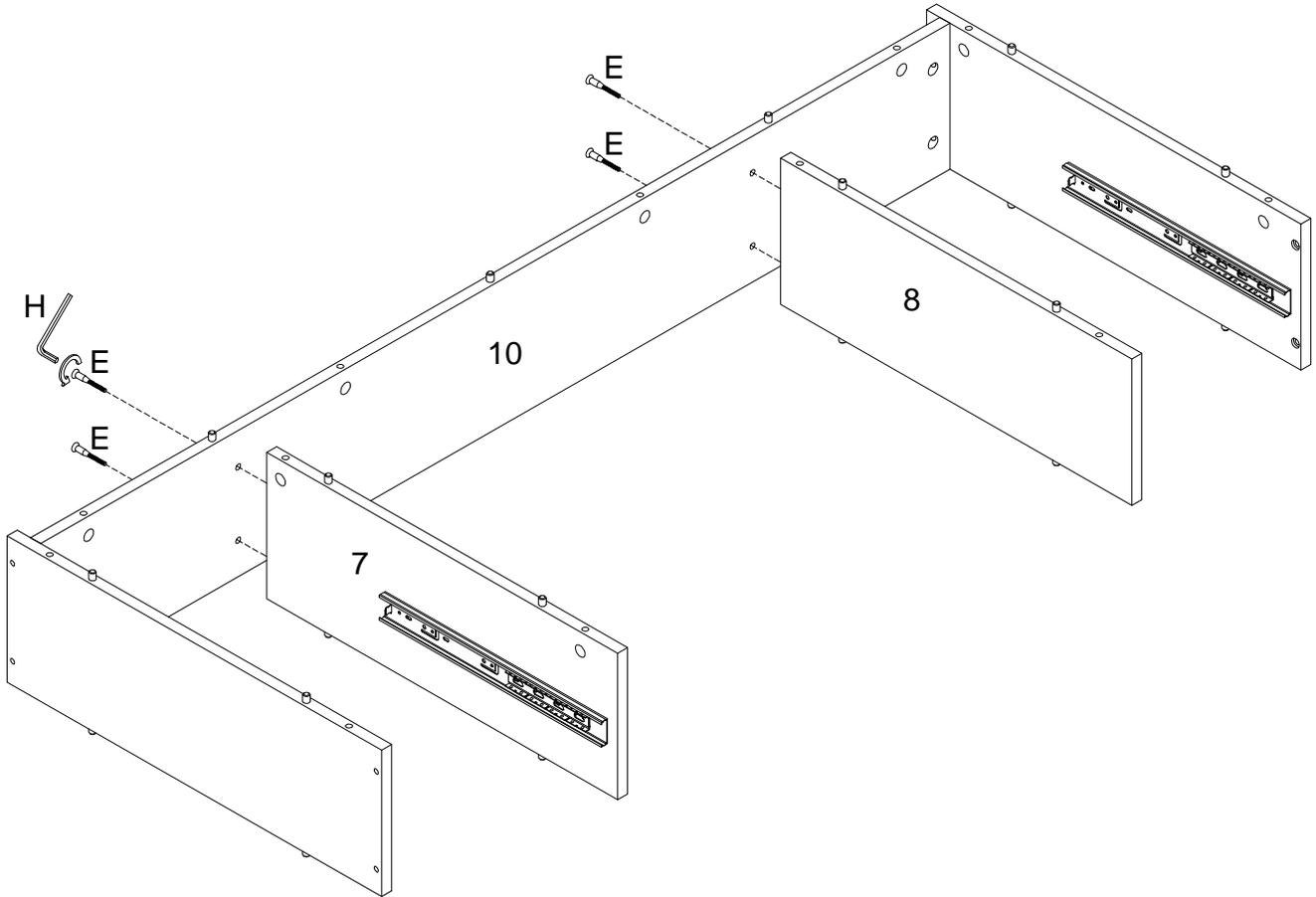
Using screw (E) attach part (10) into parts (7,8) with hex key (H) as per diagram.
