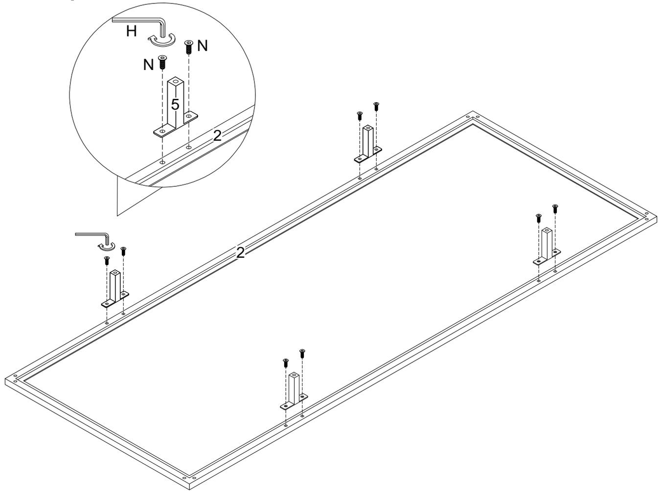
Using bolt (N) attach part (5) into part (2) with hex key (H) as per diagram.
