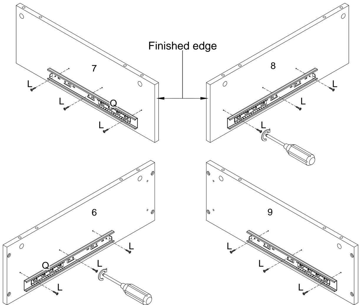
Use screw (L) attach slider (Q) into parts (6,7,8,9),with Philips head screwdriver as per diagram.
