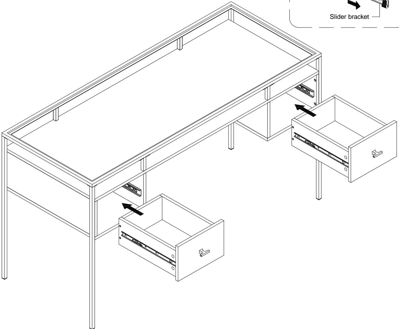
Insert the assembled drawers into the unit frame, extend the Ball Bearing Slide Tracks on the pedestal Side Panel all the way forward. Then align the Slide Runners on the assembled drawers with the Slide Tracks and push the drawer carefully inside until it stops.
