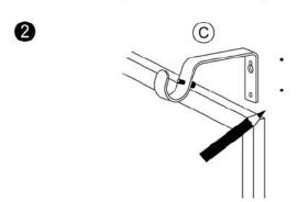
Use bracket (C) as a guide to mark location for mounting screws (A).
