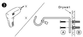
Drill pilot holes into wall with 1/4" drill bit (not included). Insert wall anchors (B) and attach bracket (C) using mounting screws (A). Wall anchors may not be necessary if drilling into studs.
