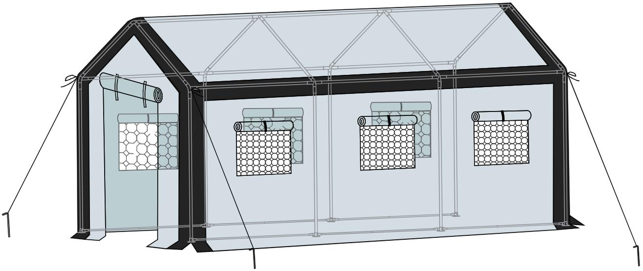
**EN\_** Be sure to always secure this greenhouse with rope attached to ground nail when in use
