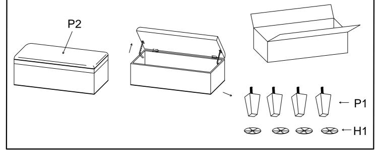
Step 2: Turn the Bench (P2) upside down and lay on soft, flat surface. Place washer (H1) onto each leg (P1), and attach the legs (P1) to the bottom of Bench (P2), Tighten each leg by turning it clockwise.
