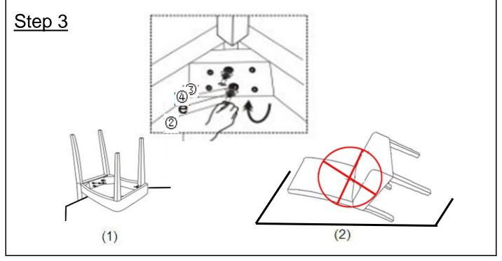
Next, place the chair onto the side of a table as seen in Picture 1. You will now have the chair bottom and all 4-legs facing skywards. Insert each front leg completely vertically into each seat frame corner. PRESS FIRMLY DOWN with your hand until there is no gap. WARNING!! DO NOT POSITION THE FRONT LEG AS SHOWN IN PICTURE 2.
