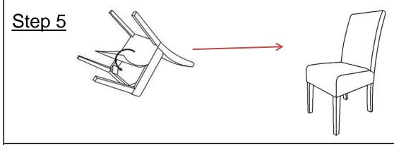
Finally, seal the Seat Base Cover back on to the underside of the chair seat . Turn it the right side up.
