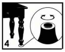
Some furniture comes with height adjusetment knobs underneath each leg. To lower or to raise each leg, you need to turn clockwise or counterclockwise, respectively.
