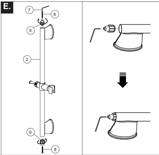
**E.** Insert an adapter (9) and screw (8) into an end of the slide bar (2). Use the included Allen wrench (7) to tighten the screw. Repeat for the other end of the slide bar.
