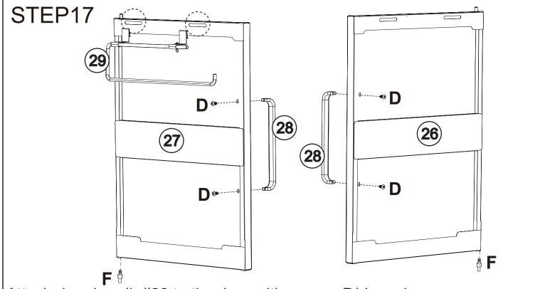
Attach door handle#28 to the door with screws D\*4 as shown.
