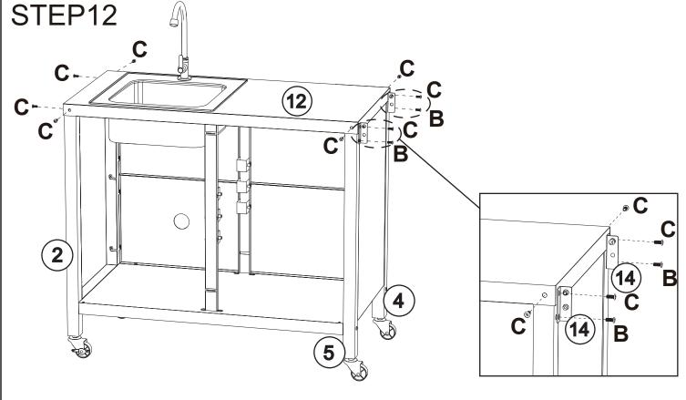
Fix the tabletop with screws C\*6 as shown. Attach Part#14 to the side at the same time with screws B\*2, C\*2 as shown.
