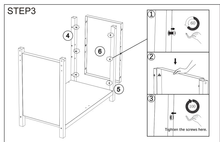
Unscrew the six screws of legs#4,#5 as shown, attach side panel #6, tighten the screws.
