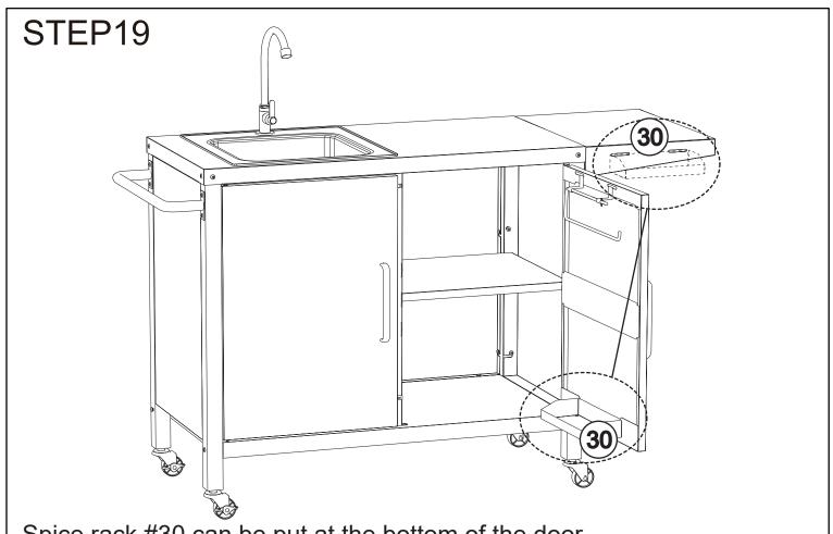
Spice rack #30 can be put at the bottom of the door, or hang on the removable panel as shown.
