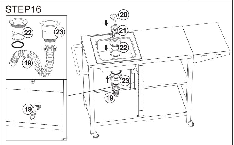
Attach part#23 to part#22 and then attach part #19 to part#23 as shown.
