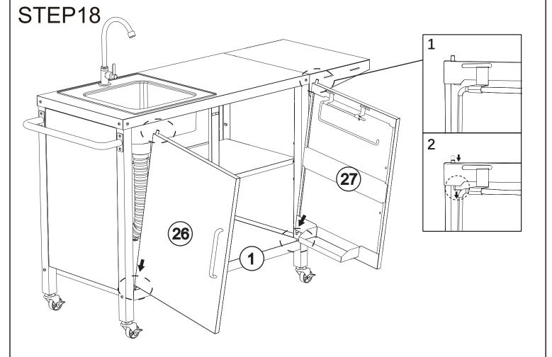
Attach the doors to the unit as shown.
