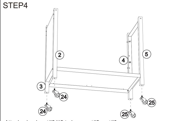
Attach wheel part#24\*2 to legs part#2,part#3. Attach wheel part#25\*2 to legs part#4,part#5 as shown.
