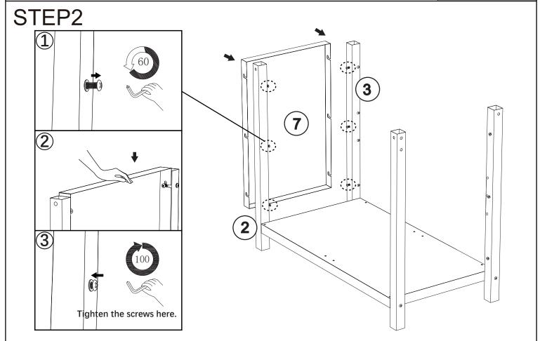
Unscrew the six screws of legs#2,#3 as shown, attach side panel #7, tighten the screws.
