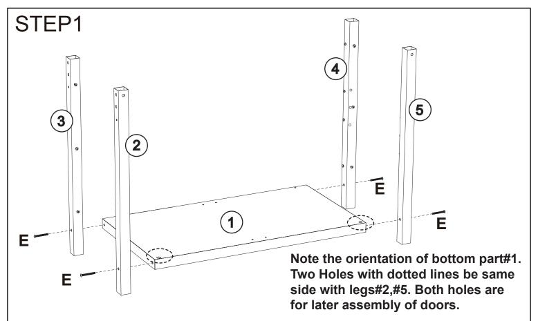
Attach Leg Parts#2,#3,#4,#5 to the bottom part#1 with screws E\*4 as shown.
