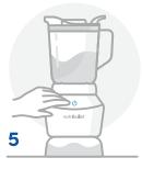
When ready, stop the appliance by pressing **POWER** (), or the function that's running, and wait for blades to stop turning.
