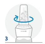
Turn the cup upside down and place it onto the motor base, gently turning clockwise to lock in place.
