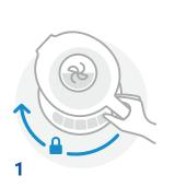
Lower the pitcher on the motor base, aligning handle on the right, and twist clockwise to lock in place.
